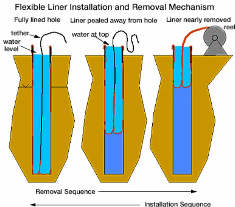
The installation of the liner is the precise reversal of this procedure. The liner is filled with water which forces it to roll out against the borehole wall as it descends into the hole. This process, the reverse of inversion, is called "eversion." By adding water and allowing the liner to pull itself to the bottom of the hole, one is back to the initial state with the liner fully extended in the hole.
